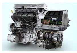
Most HEV's contain an internal combustion engine of similar size and performance to a standard combustion engined vehicle. This is needed for when rechargeable batteries that power the electric motors discharge. The combustion engine needs to be able to power the vehicle and recharge the battery packs for the electrical engine.
